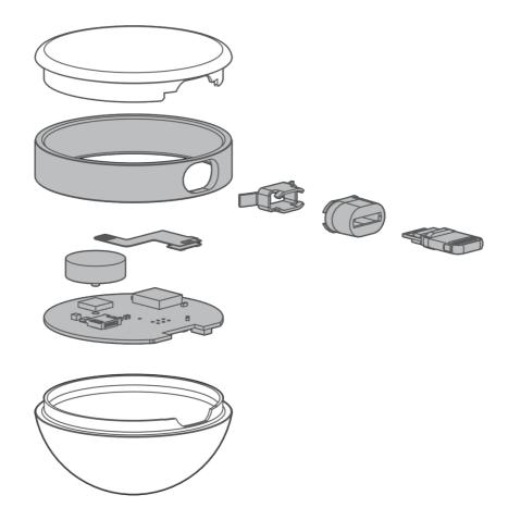
Each light meter has color sensor calibrated with 7 different light sources and photodiode calibrated for response and offsets. Calibration is automatic, each device has its own serial number, all unique raw data along with the calculated calibration constants and matrices are stored securely on the cloud servers.
