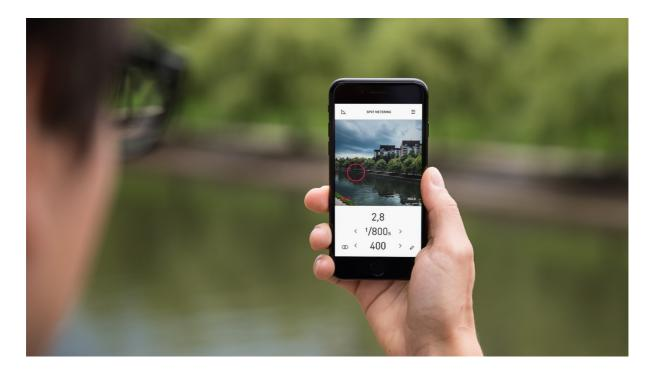
You can measure the exposure of the whole visible frame or only of a small point. When »POINT« is selected, you only measure the exposure within it's area – roughly 10° viewing angle.
