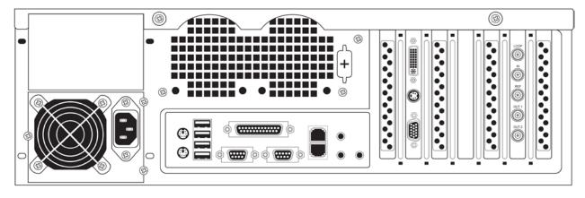
Back of 3RU server with DRC-5650 HD board installed
