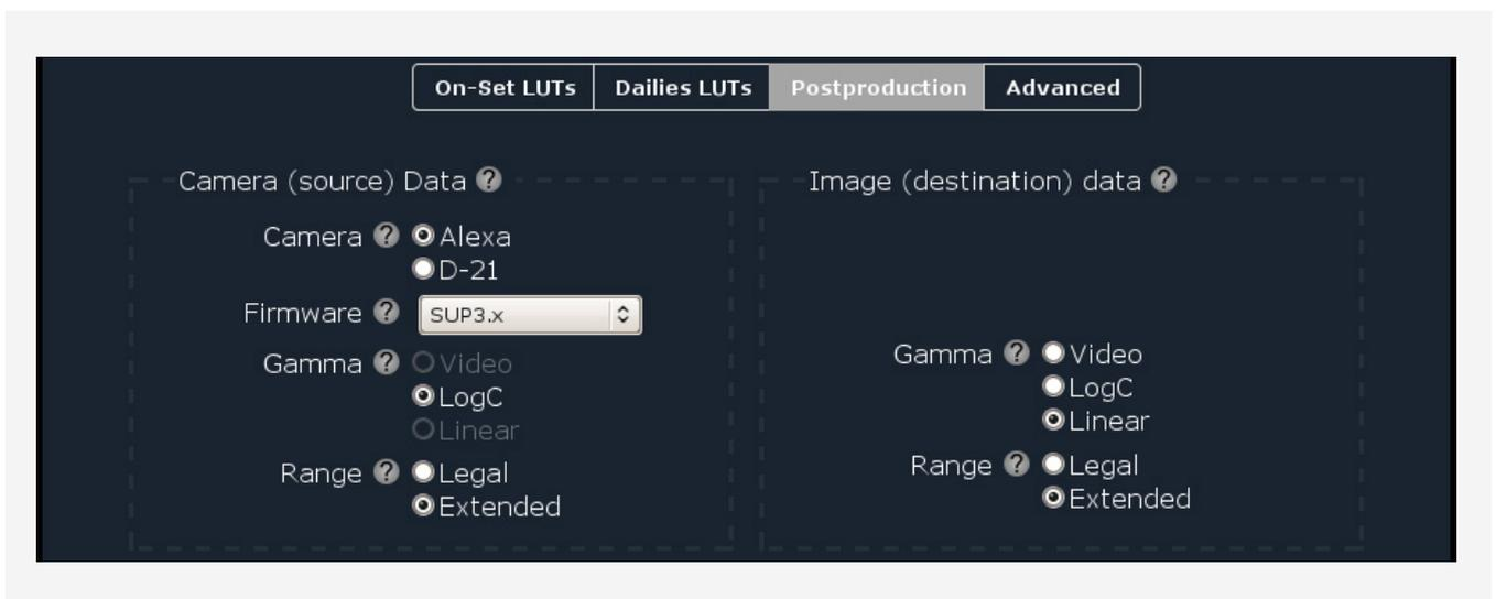
For compositing with computer generated elements images are normally converted to a linear encoding. The web application at [www.arridigital.com](http://www.arridigital.com) offers LUTs for this purpose as well.
