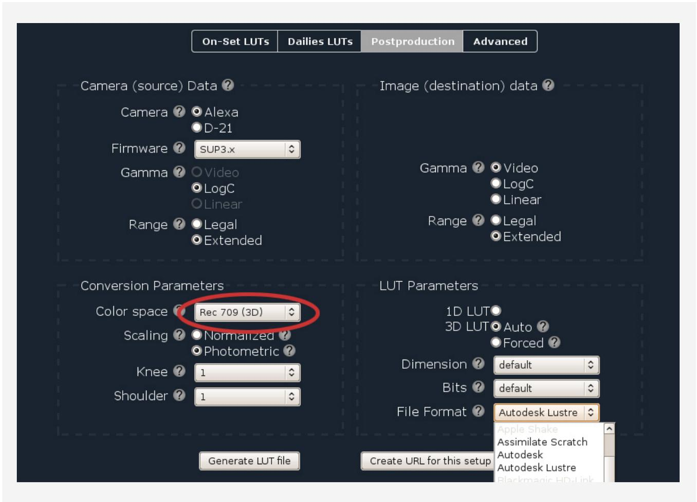
A 3DLUT is generated when a color space transformation is selected like in the example below. Note that some systems do not support 3DLUTs and are disabled in the format menu.
